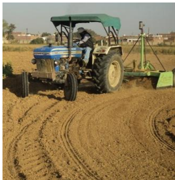
Fig 3: Shaping of field ±2 cm at 100m by laser-assist precision land leveller
