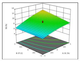
Fig 2: Response surface showing the effect of SC and ST on Solute Gain
