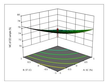
Fig 3: Response surface showing the effect of SC and ST on MC of OD sample
