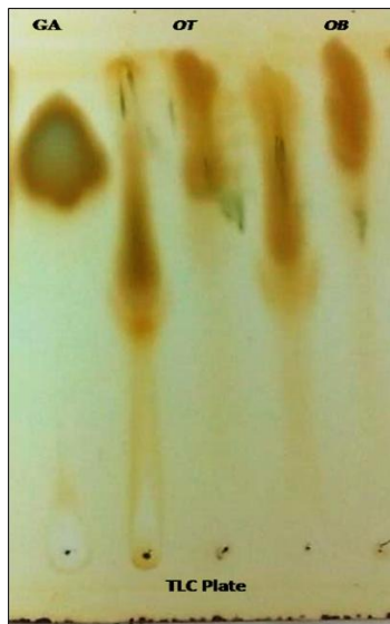
Fig 1: TLC plate showing the presence of phenols
