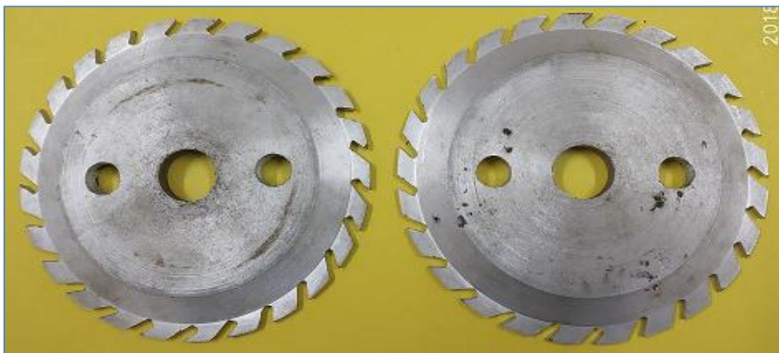
**Fig 2:** Newly fabricated metering plate
