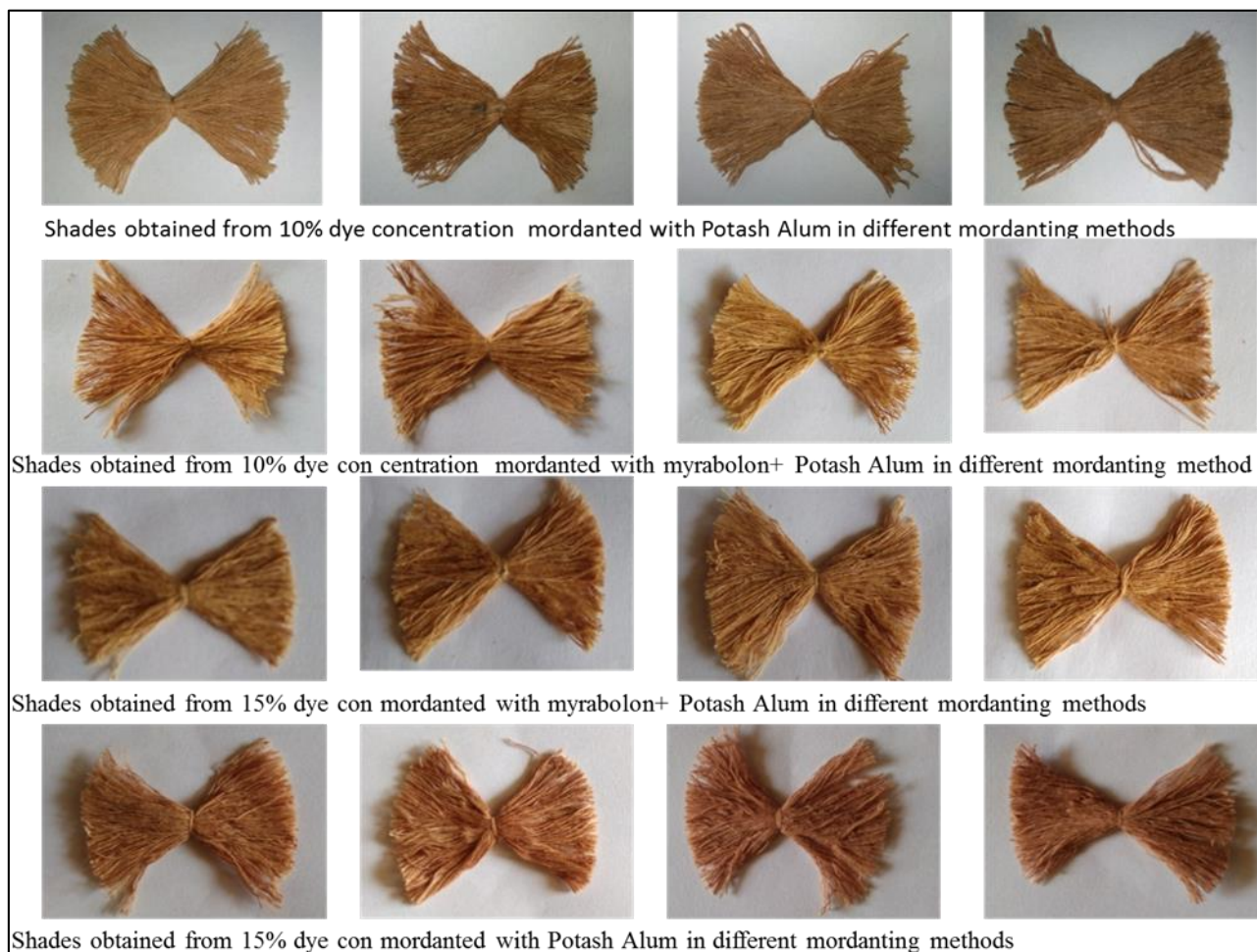
Fig 1: Shades of organic cotton dyed with dyed with Terminalia arjuna bark with different dye concentrations
