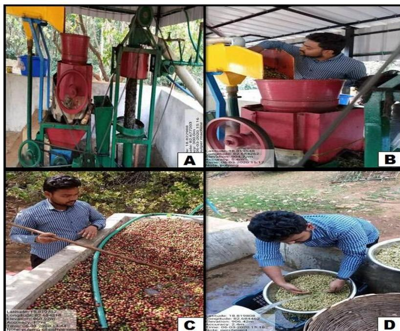
**Fig 3:** Different coffee plant operations (A) Pulper machine (B) pulping operation (C) fruits feeding to pulper (D) collection of parchment
