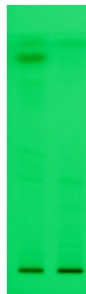
Fig 1b: Developed HPTLC plate prior to derivatization under UV 254 nm
