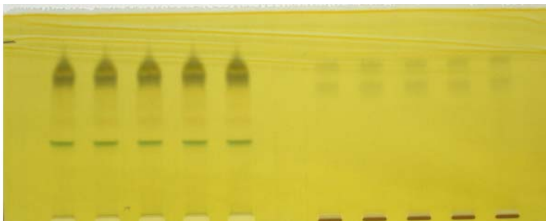
Fig 2: Alkaloid confirmation at visible, derivatisation with modified Dragendorff reagent
