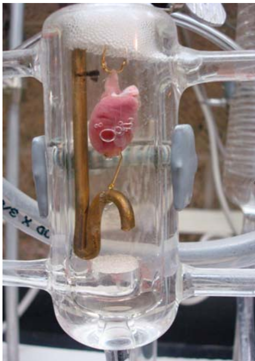
Fig 1: A rat heart anchored to a force transducer in an organ bath. The top hook is attached through an atrium, and tied to a force transducer (not pictured). The bottom hook is attached to the ventricular apex and secured to a brass bar. The bubbles at the top of the organ bath are an indication of the saponin constituent found in blue cohosh. (Photo courtesy of Joshua Hulst)
