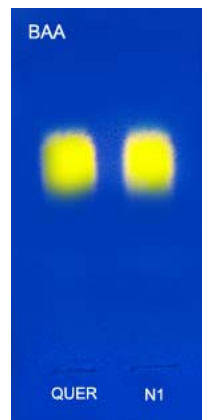
Fig 10: Characterization of quercetin by TLC (Mobile phase butanol: acetic acid: water 6:1:2)
