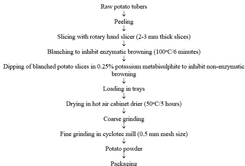
**Fig 1:** Flow chart for the preparation of potato flour
