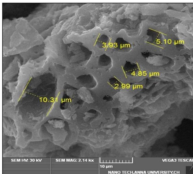
**Fig 2:** SEM Image of Coconut Shell Bio-Char
