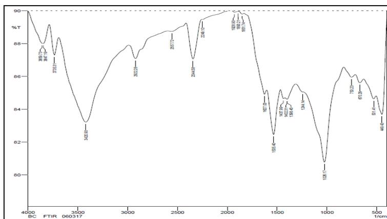
Fig 1: FT – IR of Coconut Shell Bio-Char
