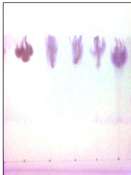
Fig 3: Detection of Phloroglucinol by thin-layer Silica Gel chromatography using n-Butanol: water: acetic acid (4:1:5), vol/vol solvent system, visualized by UV irradiation at 254 nm (Lane 1, standard Phloroglucinol; lane2, antimetabolite from isolate 379; lane 3, antimetabolite from isolate 381; lane 4, antimetabolite from isolate 384; lane 5, antimetabolite from isolate 385)
