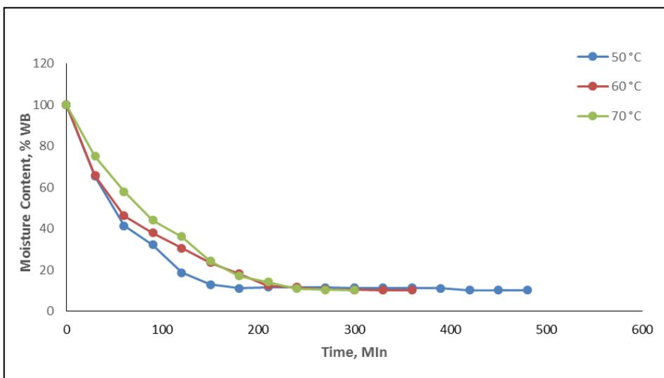
Fig 1: Time of drying vs moisture content for un-blanch samples
