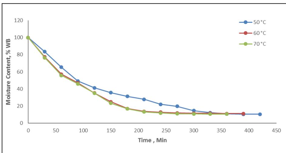
Fig 2: Time of drying vs moisture content for blanch samples
