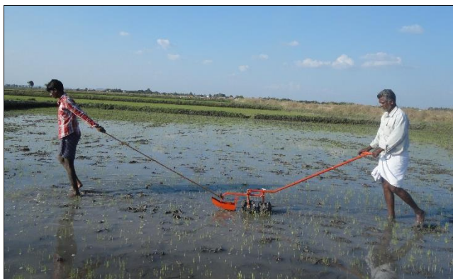
Fig 3: Schematic view of weeding operation by push type cono weeder for paddy crop
