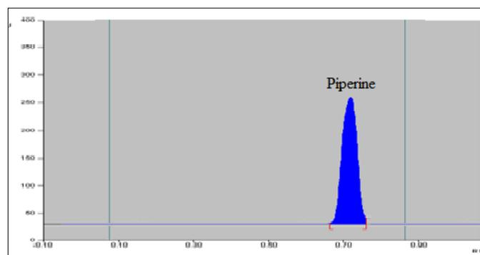
**Fig 1:** Chromatogram of standard piperine (1600 ng spot<sup>-1</sup>), ( $R_f = 0.70 \pm 0.02$ ), mobile phase: toluene: ethyl acetate: formic acid (4.8:4:0.5, v/v/v)
