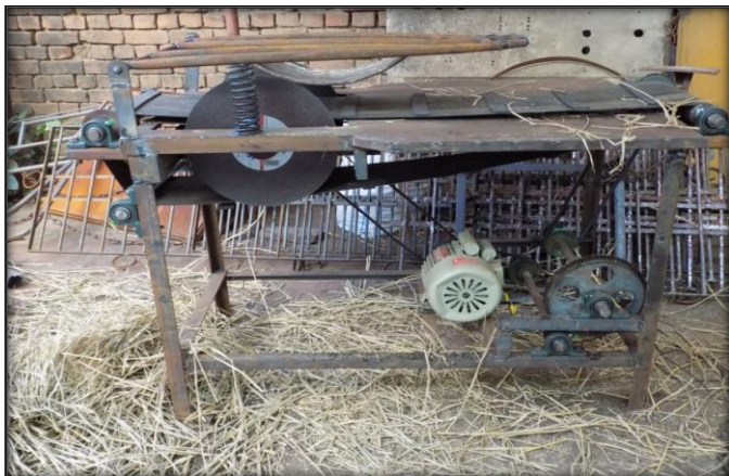
Fig 6: Straw size cutter machine after fabrication
