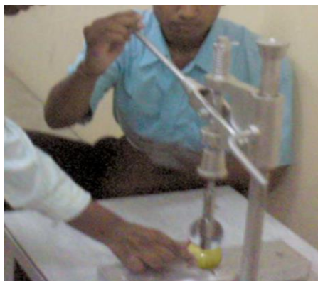
Fig 4: Manually operated aonla stone removing cum pulp slicing equipment while working
