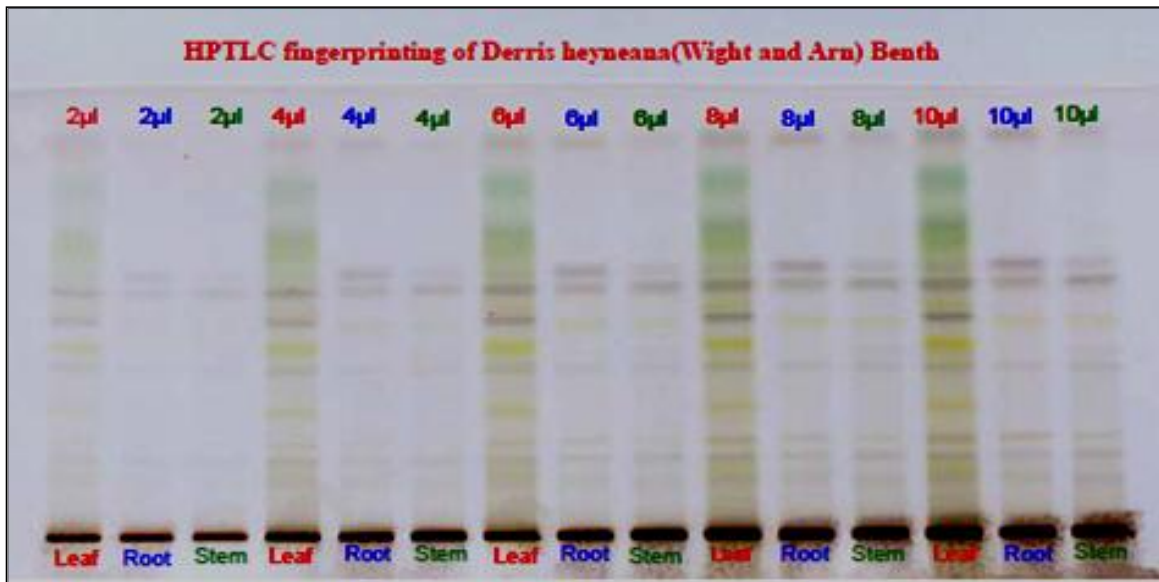
Plate 2: HPTLC fingerprint profile of Methanolic extract of leaf, root and stem of Derris heyneana (Wight and Arn) Benth. in visible light after derivatization
