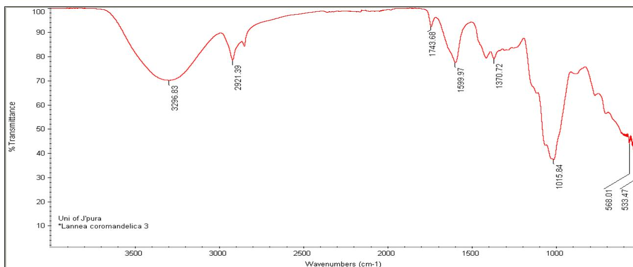
**Fig 1:** FTIR spectroscopy of Hik gum
