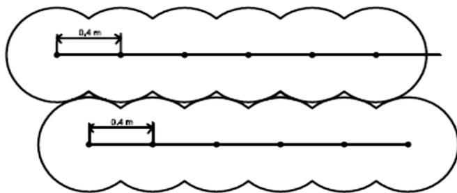
Fig 1: Triangular geometry of drip emitter
