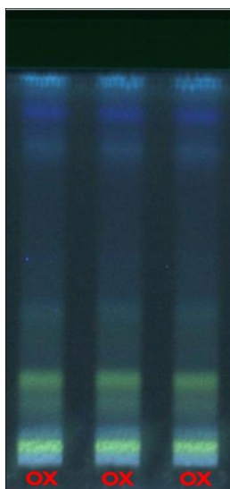
Fig 4: High performance thin layer chromatography image of Oxystelma esculentum at 366 nm in chloroform: methanol: butanol (7:2:1 v/v)
