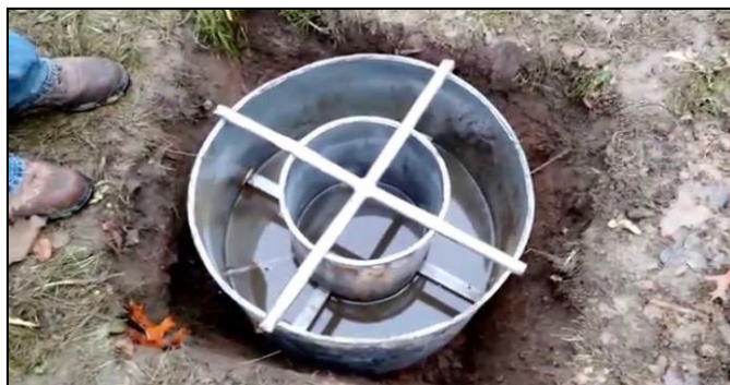
Fig 3: Double ring infiltrometer
