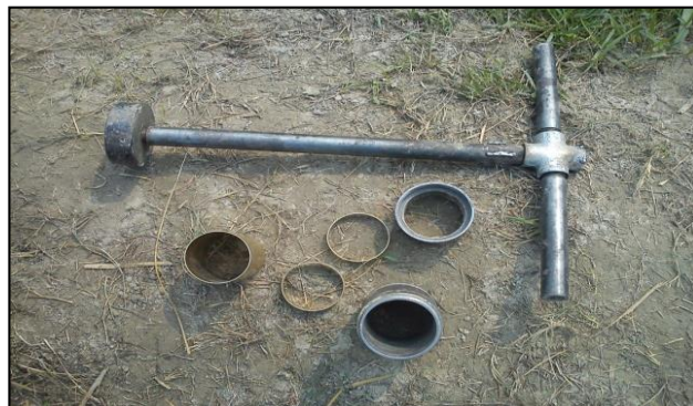
Fig 2: Core cutter soil sample
