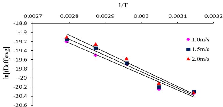
**Fig 3:** Relationship between moisture diffusivity with reciprocal of absolute temperature
