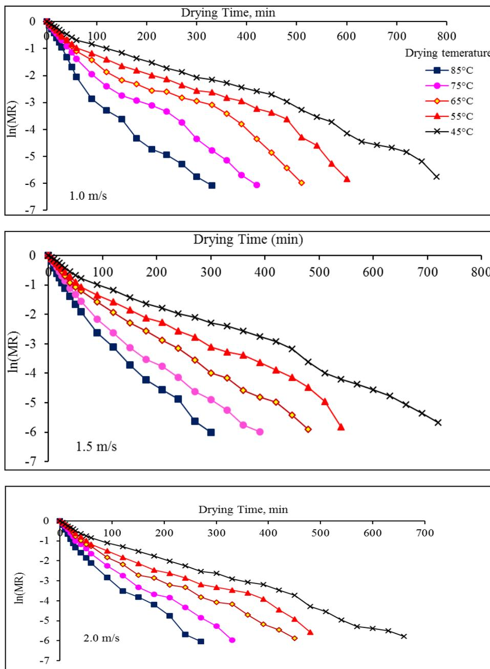
**Fig 1:** Variation in  $\ln(MR)$  versus time for convective drying of osmotically dehydrated mushroom samples
