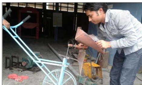
Fig 1: Fabrication of manually operated Potato earthing attachment tool.
