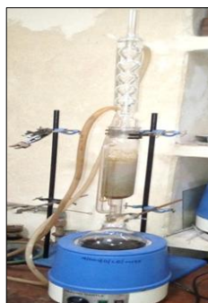
Fig 3: Soxhlet apparatus during extraction process
