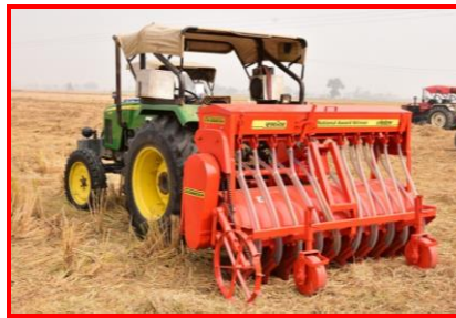
Fig 5: Happy seeder with 55 HP tractor
