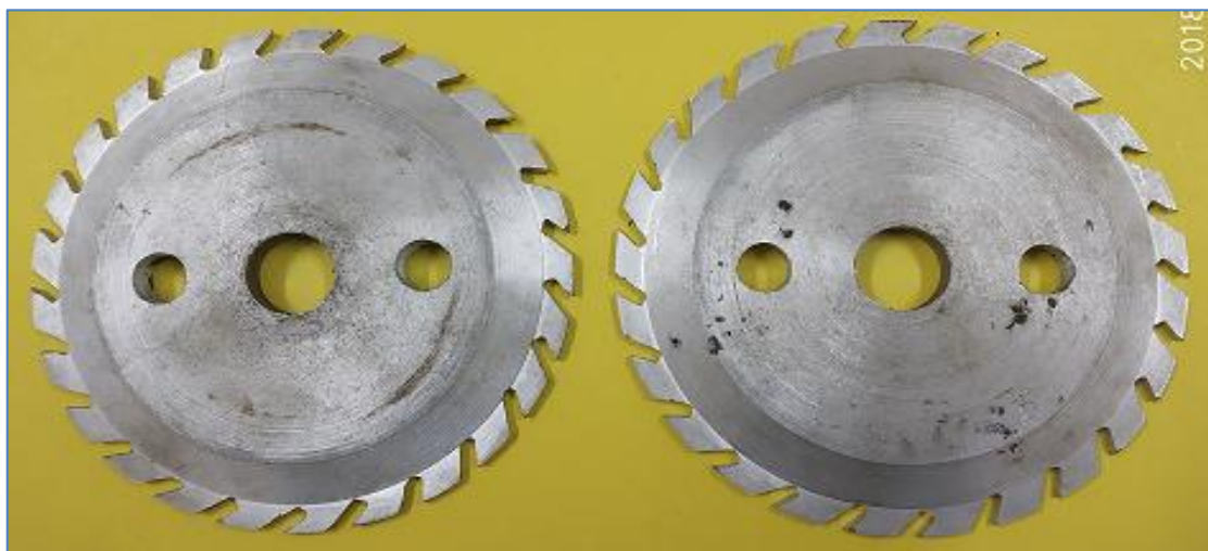
Fig 2: Newly fabricated metering plate
