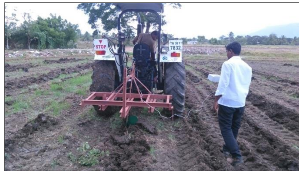
Fig 1: Draft measuring test rig in action
