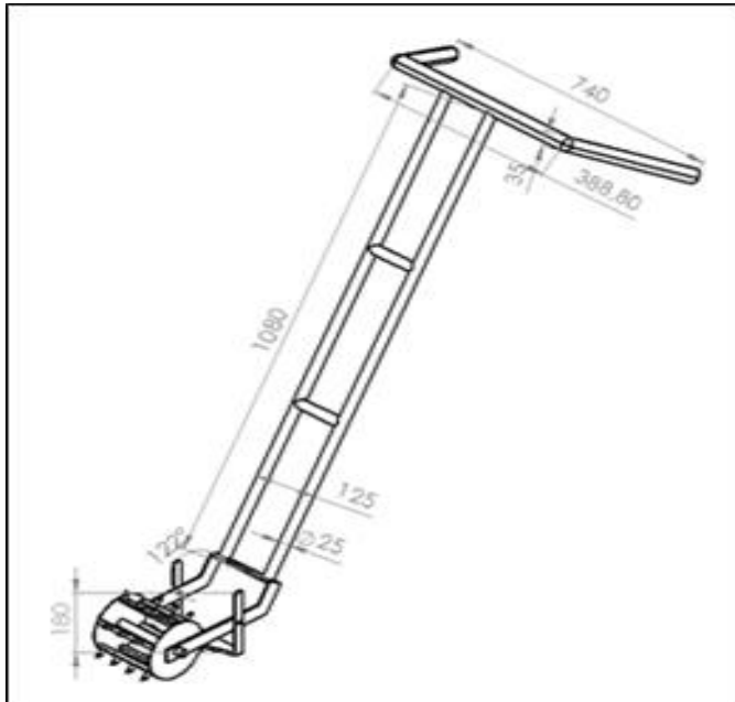
Fig 1: Schematic view of existing dry land weeder
