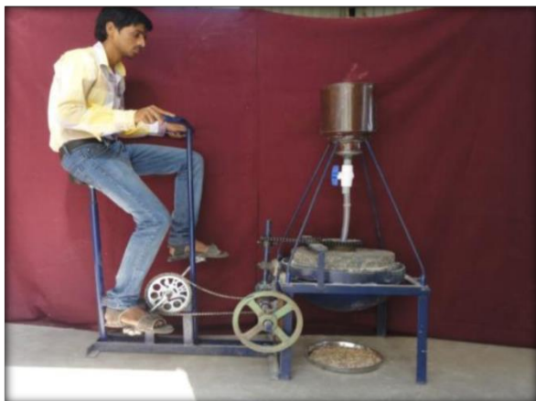
Fig 4: Heap of end product at the outlet of pedal operated flour mill
