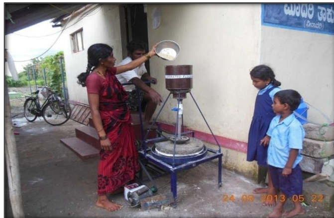
Fig 5: House hold and small poultry farmer was using pedal operated flour mill.
