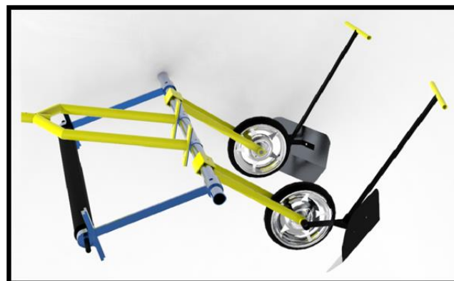
Fig 3: 3-D Solid projection of the plastic mulch laying machine
