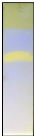
Fig 1: TLC of isolated urolithin B under UV 366 nm after treatment with 10% alcoholic KOH
