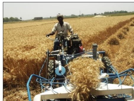
Fig 1: View of harvesting of wheat crop by Reaper-cum-binder
