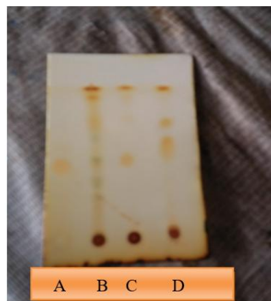
Fig 3: (A) Leaves extract (B) Bark extract, (C) Seeds extract, (D) Standard Ursolic Acid
