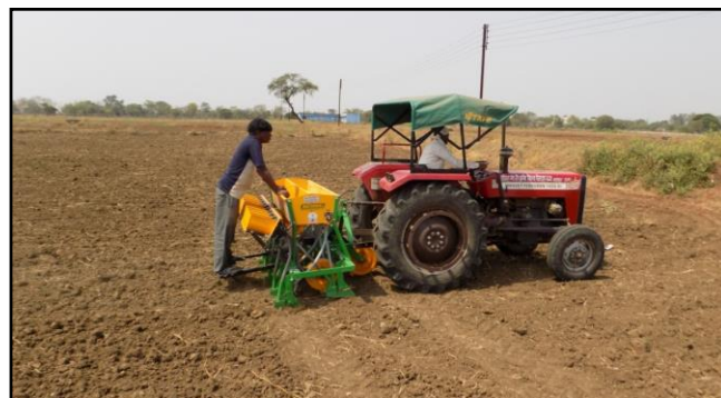
Fig 2: Field evaluations of inclined seed metering mechanism for paddy seeds
