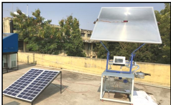
Plate 1: Experimental set-up dual axis FLSC system
