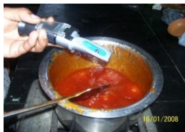
Checking the endpoint
