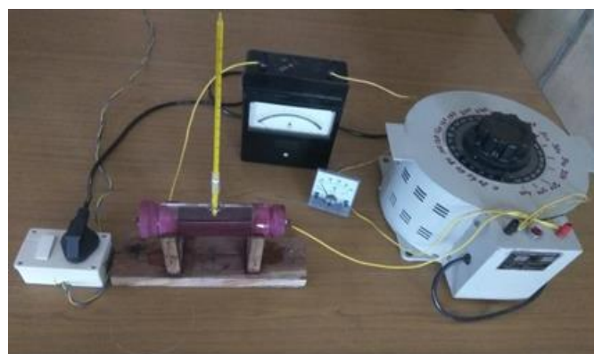
Fig 2: Pasteurization of grape juice by ohmic heating
