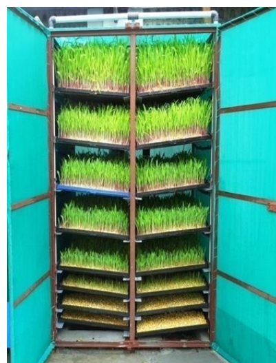
Fig 4: Trays with germinated seeds placed in the TANUVAS – UIIC – Low cost hydroponic green fodder machine
