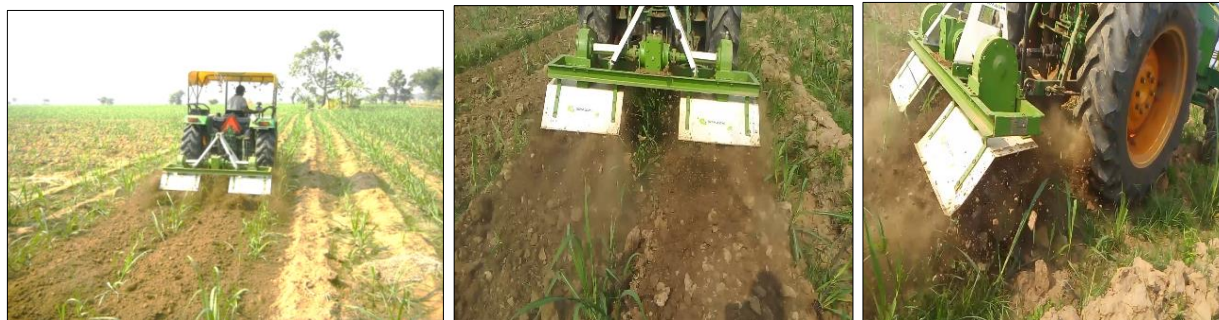
Fig 3: Field testing of tractor operated two row rotary weeder.
