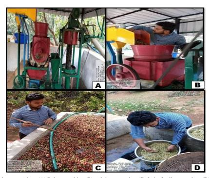
Fig 3: Different coffee plant operations (A) Pulper machine (B) pulping operation (C) fruits feeding to pulper (D) collection of parchment
