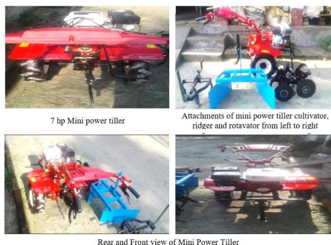
Fig 2: Mini power tiller different attachments with rear and front view
