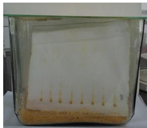
Fig 2: Iodine Chamber used for the detection in Preparative Thin Layer Chromatography
