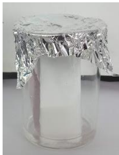
Fig 1: Pictorial representation of Real-time TLC developing chamber
