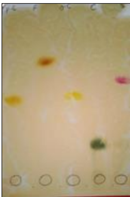
(Spot1- p -Coumaric acid, Spot2- Ferulic acid, Spot3- o -Coumaric acid, Spot4- Caffeic acid, Spot5-Sinapic acid)
