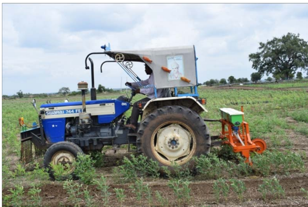
Fig 3: Field evaluation of inter-row weeder cum fertilizer applicator in redgram field
