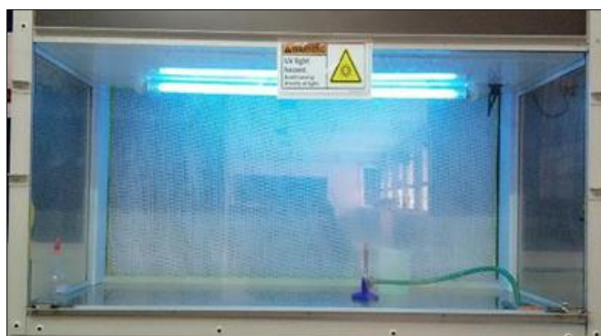
Plate 1: UV-C chamber used for sterilization of carrots
