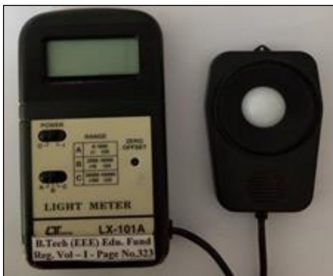
Plate 2: Hand held digital lux-meter
