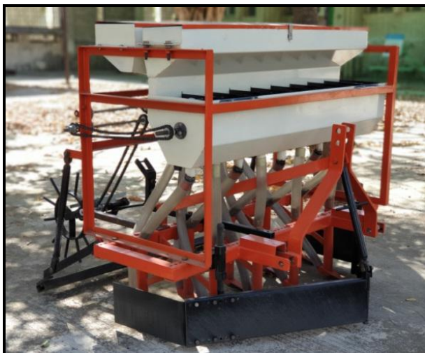
Fig 1: Prototype of developed garlic ( Allium sativum L.) clove planter
