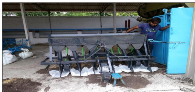
Fig 1: Laboratory calibration of prototype vermicompost subsurface manure and seed applicator
