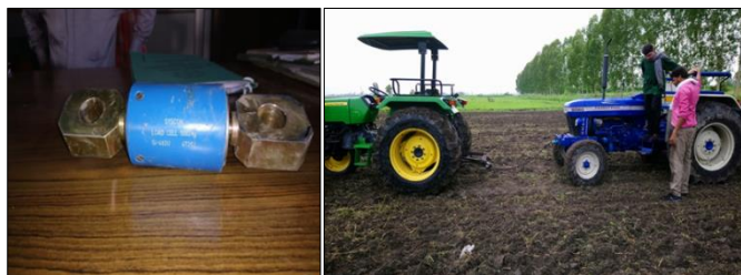
Fig 5: Draft measurement with strain gauge type load cell
