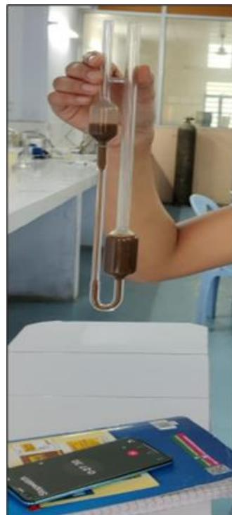
**Fig 12:** Viscosity testing using Ostwald's Viscometer
