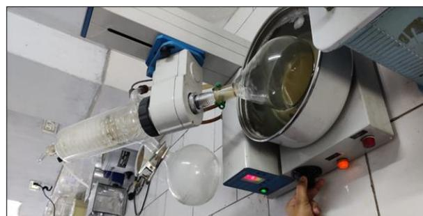
**Fig 3:** Separation process of neem extract using Rotary Evaporator
