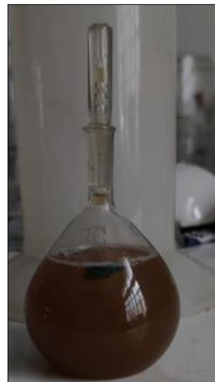
**Fig 13:** Density testing
