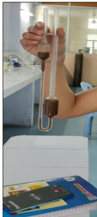
**Fig 12:** Viscosity testing using Ostwald's Viscometer
